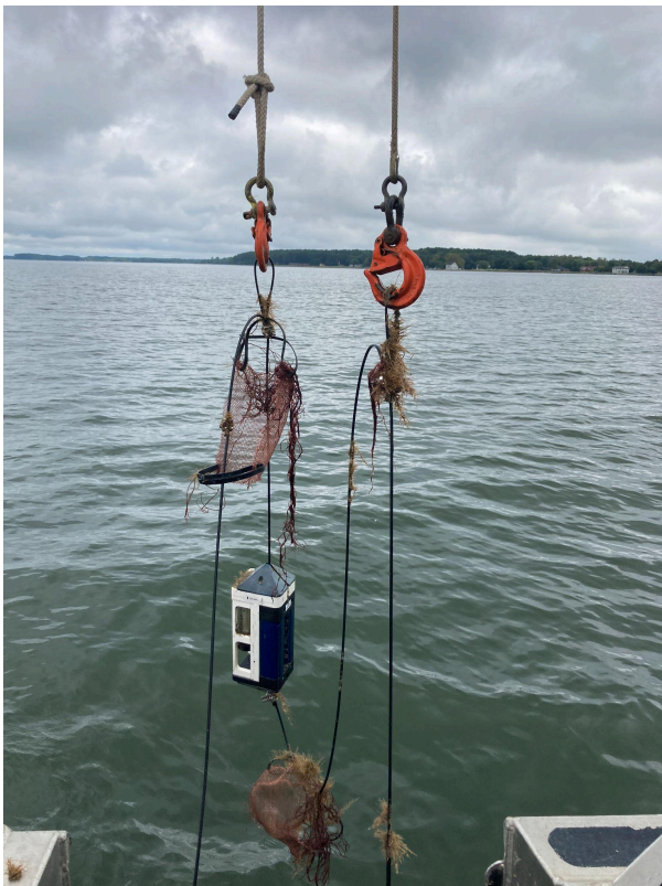
Image 4: Static line on the left holds the weight of the inductive cable plus hypoxia array while the line on the right lifts the buoy up to the vessel.
