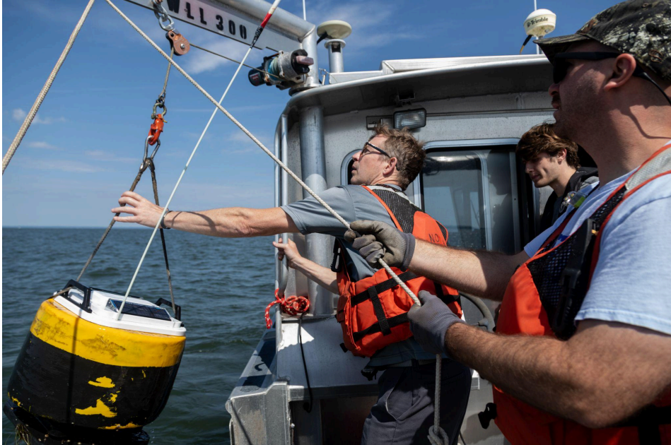
Image 3: NOAA scientists use a davit and electric motor to lift a buoy from the water.
