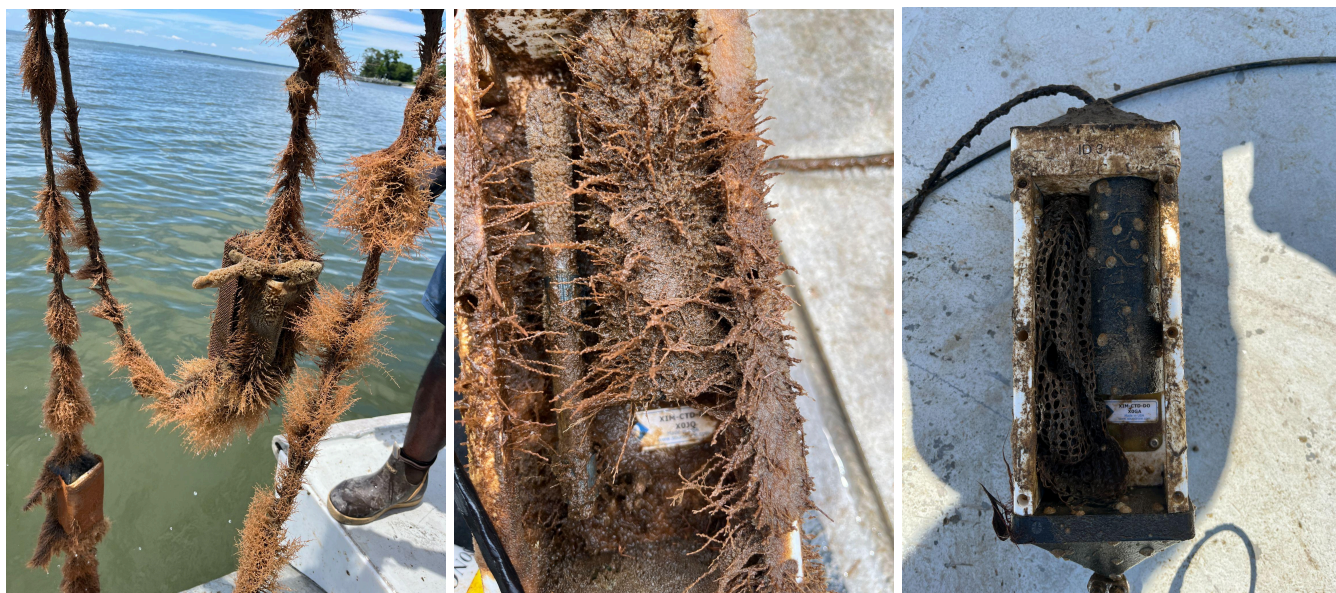
Images 3, 4, and 5: Types of biofouling observed throughout the season. Images on the left and middle show various algae growth while the image on the right side shows barnacles growing on the sensor.
