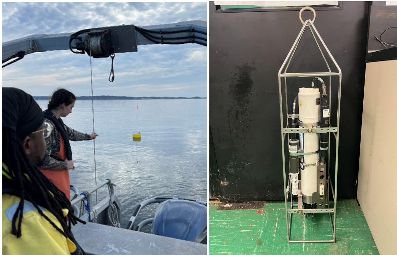
Images 6 and 7: CTD-DO being lowered into the water upon station arrival (left). Recently calibrated CTD-DO (right).
